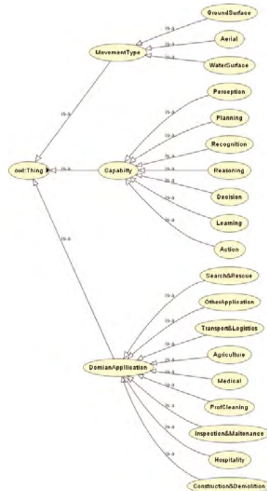
Figure 7: Categorization by movement type, capacity, and domain
